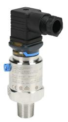
Endress+Hauser Cerabar pressure transmitter, 0 to 600 psig range, +/- 0.5% accuracy, ceramic sensing element, FKM seal(s), 4-20 mA analog output, 1/2in male NPT or 1/4in female NPT process connection, 10-30 VDC operating voltage, ISO4400 valve plug.
