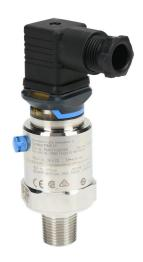
Endress+Hauser Cerabar pressure transmitter, 0 to 375 psig range, +/-0.5% accuracy, ceramic sensing element, FKM seal(s), 4-20 mA analog output, 1/2in male NPT or 1/4in female NPT process connection, 10 to 30 VDC operating voltage, ISO4400 valve plug.
