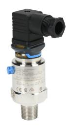
Endress+Hauser Cerabar pressure transmitter, 0 to 375 psig range, +/- 0.5% accuracy, ceramic sensing element, FKM seal(s), 4-20 mA analog output, 1/2in male NPT or 1/4in female NPT process connection, 10-30 VDC operating voltage, ISO4400 valve plug.
