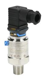
Endress+Hauser Cerabar pressure transmitter, 0 to 150 psig range, +/- 0.5% accuracy, ceramic sensing element, FKM seal(s), 4-20 mA analog output, 1/2in male NPT or 1/4in female NPT process connection, 10-30 VDC operating voltage, ISO4400 valve plug.
