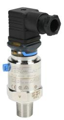
Endress+Hauser Cerabar pressure transmitter, 0 to 90 psig range, +/- 0.5% accuracy, ceramic sensing element, FKM seal(s), 4-20 mA analog output, 1/2in male NPT or 1/4in female NPT process connection, 10-30 VDC operating voltage, ISO4400 valve plug.
