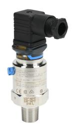
Endress+Hauser Cerabar pressure transmitter, 0 to 60 psig range, +/- 0.5% accuracy, ceramic sensing element, FKM seal(s), 4-20 mA analog output, 1/2in male NPT or 1/4in female NPT process connection, 10-30 VDC operating voltage, ISO4400 valve plug.
