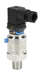
Endress+Hauser Cerabar pressure transmitter, 0 to 30 psig range, +/- 0.5% accuracy, ceramic sensing element, FKM seal(s), 4-20 mA analog output, 1/2in male NPT or 1/4in female NPT process connection, 10-30 VDC operating voltage, ISO4400 valve plug.
