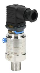
Endress+Hauser Cerabar pressure transmitter, 0 to 6 psig range, +/- 0.5% accuracy, ceramic sensing element, FKM seal(s), 4-20 mA analog output, 1/2in male NPT or 1/4in female NPT process connection, 10-30 VDC operating voltage, ISO4400 valve plug.
