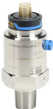
Endress+Hauser Cerabar pressure transmitter, 0 to 600 psig range, +/- 0.5% accuracy, ceramic sensing element, FKM seal(s), 4-20 mA analog output, 1/2in male NPT or 1/4in female NPT process connection, 10-30 VDC operating voltage, 4-pin M12 quick-disconnect.
