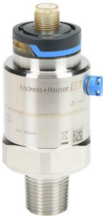
Endress+Hauser Cerabar pressure transmitter, 0 to 150 psig range, +/-0.5% accuracy, ceramic sensing element, FKM seal(s), 4-20 mA analog output, 1/2in male NPT or 1/4in female NPT process connection, 10 to 30 VDC operating voltage, 4-pin M12 quick-disconnect.
