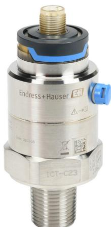
Endress+Hauser Cerabar pressure transmitter, 0 to 30 psig range, +/- 0.5% accuracy, ceramic sensing element, FKM seal(s), 4-20 mA analog output, 1/2in male NPT or 1/4in female NPT process connection, 10-30 VDC operating voltage, 4-pin M12 quick-disconnect.
