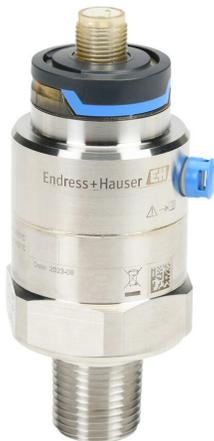
Endress+Hauser Cerabar pressure transmitter, 0 to 15 psig range, +/- 0.5% accuracy, ceramic sensing element, FKM seal(s), 4-20 mA analog output, 1/2in male NPT or 1/4in female NPT process connection, 10-30 VDC operating voltage, 4-pin M12 quick-disconnect.
