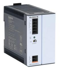
BLOCK Power Mini series switching power supply, 24 VDC @ 4A/96W (adjustable), 100-240 VAC nominal input, 1-phase, enclosed, plastic housing, 35mm DIN rail mount, push terminals.
