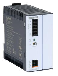
BLOCK Power Mini series switching power supply, 24 VDC @ 2A/48W (adjustable), 100-240 VAC nominal input, 1-phase, enclosed, plastic housing, 35mm DIN rail mount, push terminals, NEC Class 2.
