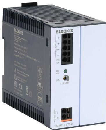
BLOCK Power Mini series switching power supply, 12 VDC @ 7A/84W (adjustable), 100-240 VAC nominal input, 1-phase, enclosed, plastic housing, 35mm DIN rail mount, push terminals.
