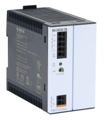
BLOCK Power Mini series switching power supply, 12 VDC @ 7A/84W (adjustable), 100-240 VAC nominal input, 1-phase, enclosed, plastic housing, 35mm DIN rail mount, push terminals.
