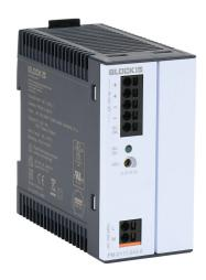
BLOCK Power Mini series switching power supply, 12 VDC @ 4A/48W (adjustable), 100-240 VAC nominal input, 1-phase, enclosed, plastic housing, 35mm DIN rail mount, push terminals, NEC Class 2.
