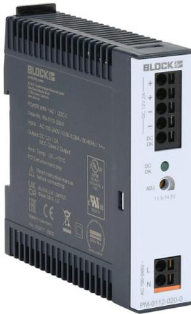
BLOCK Power Mini series switching power supply, 12 VDC @ 2A/24W (adjustable), 100-240 VAC nominal input, 1-phase, enclosed, plastic housing, 35mm DIN rail mount, push terminals, NEC Class 2.
