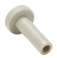
HydroMode potable water push-to-connect fitting, plug, acetal body, (1) 1/4in plug-in connection(s), NSF/ANSI 61. Package of 5.
