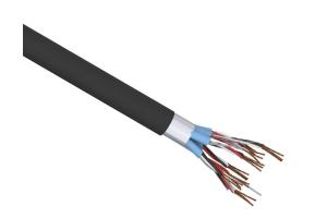
Quabbin instrumentation cable, individual and overall shielded, PLTC and ITC, 300V, 8 twisted triads, 20 AWG, PVC conductor insulation material, black, white and red, PVC jacket, black, cut to length.
