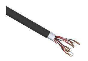
Quabbin instrumentation cable, overall shielded, PLTC and ITC, 300V, 8 twisted triads, 20 AWG, PVC conductor insulation material, black, white and red, PVC jacket, black, cut to length.
