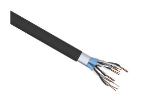
Quabbin instrumentation cable, individual and overall shielded, PLTC, 300V, 8 twisted pairs, 20 AWG, PVC conductor insulation material, black and white numbered pairs, PVC jacket, black, cut to length.
