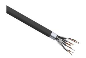
Quabbin instrumentation cable, overall shielded, PLTC, 300V, 8 twisted pairs, 20 AWG, PVC conductor insulation material, black and white numbered pairs, PVC jacket, black, cut to length.
