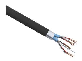
Quabbin instrumentation cable, individual and overall shielded, PLTC and ITC, 300V, 4 twisted triads, 20 AWG, PVC conductor insulation material, black, white and red, PVC jacket, black, cut to length.
