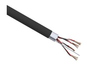
Quabbin instrumentation cable, overall shielded, PLTC and ITC, 300V, 4 twisted triads, 20 AWG, PVC conductor insulation material, black, white and red, PVC jacket, black, cut to length.
