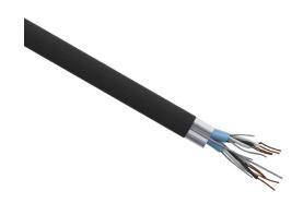
Quabbin instrumentation cable, individual and overall shielded, PLTC, 300V, 4 twisted pairs, 20 AWG, PVC conductor insulation material, black and white numbered pairs, PVC jacket, black, cut to length.
