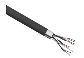
Quabbin instrumentation cable, overall shielded, PLTC, 300V, 4 twisted pairs, 20 AWG, PVC conductor insulation material, black and white numbered pairs, PVC jacket, black, cut to length.
