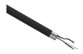
Quabbin instrumentation cable, overall shielded, PLTC and ITC, 300V, 2 twisted triads, 20 AWG, PVC conductor insulation material, black, white and red, PVC jacket, black, cut to length.
