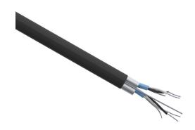
Quabbin instrumentation cable, individual and overall shielded, PLTC, 300V, 2 twisted pairs, 20 AWG, PVC conductor insulation material, black and white numbered pairs, PVC jacket, black, cut to length.
