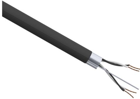
Quabbin instrumentation cable, overall shielded, PLTC, 300V, 2 twisted pairs, 20 AWG, PVC conductor insulation material, black and white numbered pairs, PVC jacket, black, cut to length.
