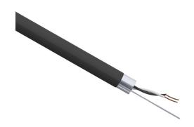
Quabbin instrumentation cable, overall shielded, PLTC, 300V, 1 twisted pair, 20 AWG, PVC conductor insulation material, black and white numbered pairs, PVC jacket, black, cut to length.
