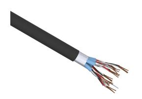
Quabbin instrumentation cable, individual and overall shielded, PLTC and ITC, 300V, 8 twisted triads, 18 AWG, PVC conductor insulation material, black, white and red, PVC jacket, black, cut to length.
