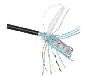
Southwire instrumentation cable, individual and overall shielded, PLTC and ITC, 300V, 8 twisted pairs, 18 AWG, PVC conductor insulation material, black and white numbered pairs, PVC jacket, black, cut to length.
