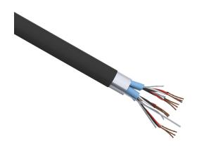
Quabbin instrumentation cable, individual and overall shielded, PLTC and ITC, 300V, 4 twisted triads, 18 AWG, PVC conductor insulation material, black, white and red, PVC jacket, black, cut to length.
