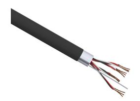
Quabbin instrumentation cable, overall shielded, PLTC and ITC, 300V, 4 twisted triads, 18 AWG, PVC conductor insulation material, black, white and red, PVC jacket, black, cut to length.
