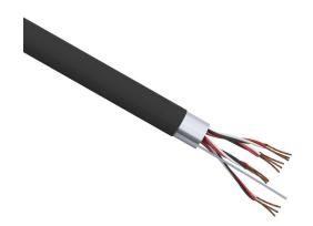
Quabbin instrumentation cable, overall shielded, PLTC and ITC, 300V, 4 twisted triads, 18 AWG, PVC conductor insulation material, black, white and red, PVC jacket, black, cut to length.
