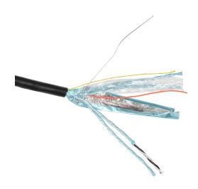
Southwire instrumentation cable, individual and overall shielded, PLTC and ITC, 300V, 4 twisted pairs, 18 AWG, PVC conductor insulation material, black and white numbered pairs, PVC jacket, black, cut to length.
