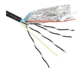
Southwire instrumentation cable, overall shielded, PLTC and ITC, 300V, 4 twisted pairs, 18 AWG, PVC conductor insulation material, black and white numbered pairs, PVC jacket, black, cut to length.
