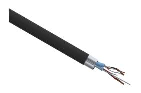
Quabbin instrumentation cable, individual and overall shielded, PLTC and ITC, 300V, 2 twisted triads, 18 AWG, PVC conductor insulation material, black, white and red, PVC jacket, black, cut to length.
