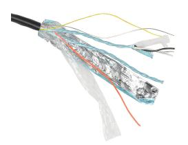
Southwire instrumentation cable, individual and overall shielded, PLTC and ITC, 300V, 2 twisted pairs, 18 AWG, PVC conductor insulation material, black and white numbered pairs, PVC jacket, black, cut to length.
