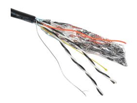
Southwire instrumentation cable, overall shielded, PLTC and ITC, 300V, 2 twisted pairs, 18 AWG, PVC conductor insulation material, black and white numbered pairs, PVC jacket, black, cut to length.
