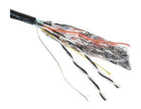
Southwire instrumentation cable, overall shielded, PLTC and ITC, 300V, 2 twisted pairs, 18 AWG, PVC conductor insulation material, black and white numbered pairs, PVC jacket, black, cut to length.
