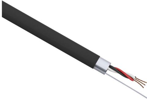
Quabbin instrumentation cable, overall shielded, PLTC and ITC, 300V, 1 twisted triad, 18 AWG, PVC conductor insulation material, black, white and red, PVC jacket, black, cut to length.
