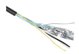
Southwire instrumentation cable, overall shielded, PLTC and ITC, 300V, 1 twisted pair, 18 AWG, PVC conductor insulation material, black and white numbered pairs, PVC jacket, black, cut to length.
