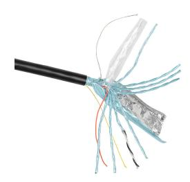
Southwire instrumentation cable, individual and overall shielded, PLTC and ITC, 300V, 8 twisted pairs, 16 AWG, PVC conductor insulation material, black and white numbered pairs, PVC jacket, black, cut to length.
