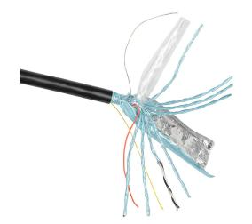
Southwire instrumentation cable, individual and overall shielded, PLTC and ITC, 300V, 8 twisted pairs, 16 AWG, PVC conductor insulation material, black and white numbered pairs, PVC jacket, black, cut to length.
