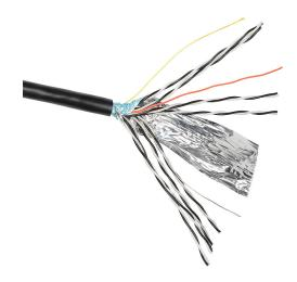
Southwire instrumentation cable, overall shielded, PLTC and ITC, 300V, 8 twisted pairs, 16 AWG, PVC conductor insulation material, black and white numbered pairs, PVC jacket, black, cut to length.
