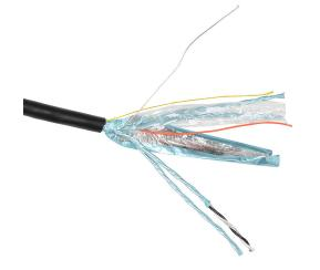
Southwire instrumentation cable, individual and overall shielded, PLTC and ITC, 300V, 4 twisted pairs, 16 AWG, PVC conductor insulation material, black and white numbered pairs, PVC jacket, black, cut to length.
