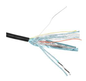
Southwire instrumentation cable, individual and overall shielded, PLTC and ITC, 300V, 4 twisted pairs, 16 AWG, PVC conductor insulation material, black and white numbered pairs, PVC jacket, black, cut to length.
