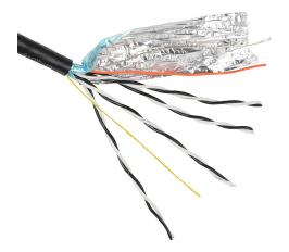
Southwire instrumentation cable, overall shielded, PLTC and ITC, 300V, 4 twisted pairs, 16 AWG, PVC conductor insulation material, black and white numbered pairs, PVC jacket, black, cut to length.
