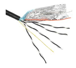
Southwire instrumentation cable, overall shielded, PLTC and ITC, 300V, 4 twisted pairs, 16 AWG, PVC conductor insulation material, black and white numbered pairs, PVC jacket, black, cut to length.
