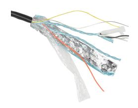
Southwire instrumentation cable, individual and overall shielded, PLTC and ITC, 300V, 2 twisted pairs, 16 AWG, PVC conductor insulation material, black and white numbered pairs, PVC jacket, black, cut to length.
