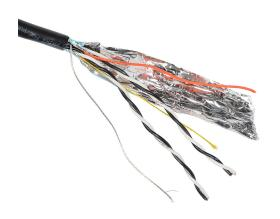
Southwire instrumentation cable, overall shielded, PLTC and ITC, 300V, 2 twisted pairs, 16 AWG, PVC conductor insulation material, black and white numbered pairs, PVC jacket, black, cut to length.
