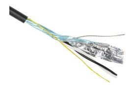
Southwire instrumentation cable, overall shielded, PLTC and ITC, 300V, 1 twisted pair, 16 AWG, PVC conductor insulation material, black and white numbered pairs, PVC jacket, black, cut to length.
