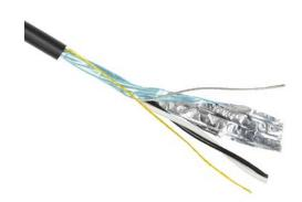
Southwire instrumentation cable, overall shielded, PLTC and ITC, 300V, 1 twisted pair, 16 AWG, PVC conductor insulation material, black and white numbered pairs, PVC jacket, black, cut to length.
