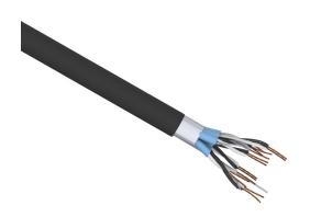
Quabbin instrumentation cable, individual and overall shielded, PLTC and ITC, 300V, 8 twisted pairs, 18 AWG, PVC conductor insulation material, black and white numbered pairs, PVC jacket, black, cut to length.
