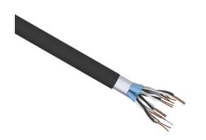
Quabbin instrumentation cable, individual and overall shielded, PLTC and ITC, 300V, 8 twisted pairs, 18 AWG, PVC conductor insulation material, black and white numbered pairs, PVC jacket, black, cut to length.
