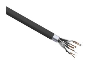
Quabbin instrumentation cable, overall shielded, PLTC and ITC, 300V, 8 twisted pairs, 18 AWG, PVC conductor insulation material, black and white numbered pairs, PVC jacket, black, cut to length.
