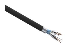
Quabbin instrumentation cable, individual and overall shielded, PLTC and ITC, 300V, 4 twisted pairs, 18 AWG, PVC conductor insulation material, black and white numbered pairs, PVC jacket, black, cut to length.
